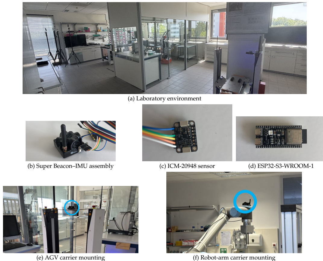
Figure 4. Photographic documentation of the experimental environment, embedded sensing hardware, and carrier mounting configurations. The ultrasonic-inertial sensing node was mounted on the AGV platform for 2D mobile tests and above the UR10 wrist joint for controlled 3D trajectory evaluation; the wrist joint was kept fixed so that the sensor-to-end-effector transform remained constant. The blue circles in (e,f) indicate the mounting positions of the sensors on the AGV and the robotic arm, respectively.
