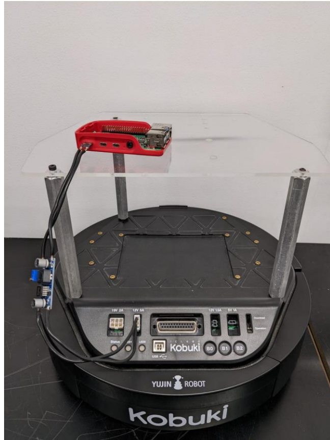
Figure 4-3: Raspberry Pi 4 Model B powered by the 12V/5A connector on Kobuki via the LM2956 Buck Converter
