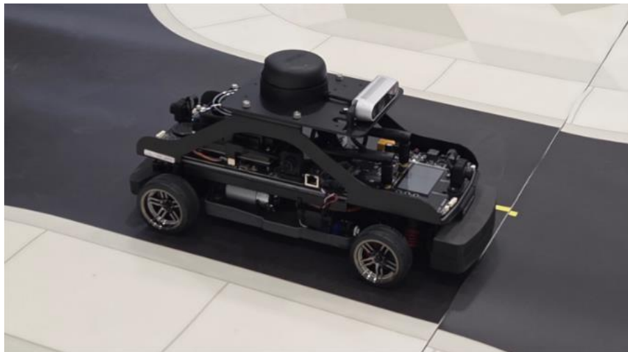
Figure 2: First Class Quanser QCar Autonomously Navigating Using Optitrack
