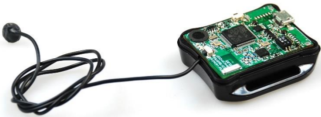
Figure 1: One external microphone with housing
