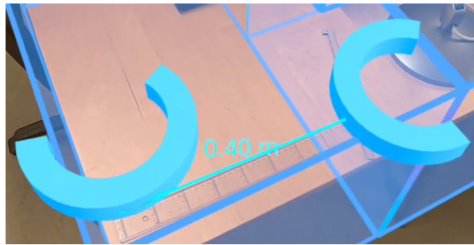
Figure 4.6 Two virtual objects on top of a 40 cm ruler, showing the virtual distance between the centre of the objects.
