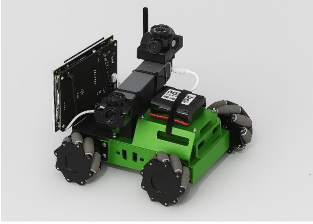
Fig. 2. Autonomous mobile robot platform equipped with four Mecanum wheels, An NVIDIA Jetson Nano, and Marvelmind indoor positioning system (IPS) beacons for indoor localization.
