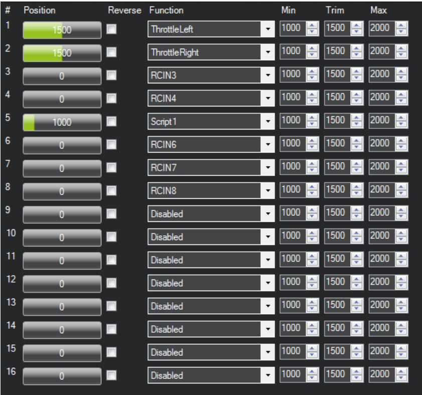
Figure 6. ArduRover servo output configuration.
